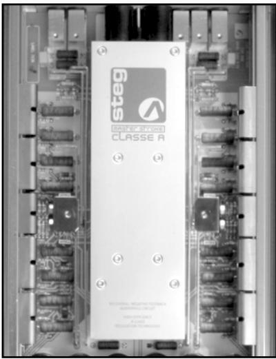
Power output stage and driver
